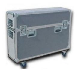
The construction of this case is 3/8" plywood sidewall, recessed handles and spring-loaded twist-lock latches, stamped nickel-plated large flat corners, key locks and 4" locking casters.
